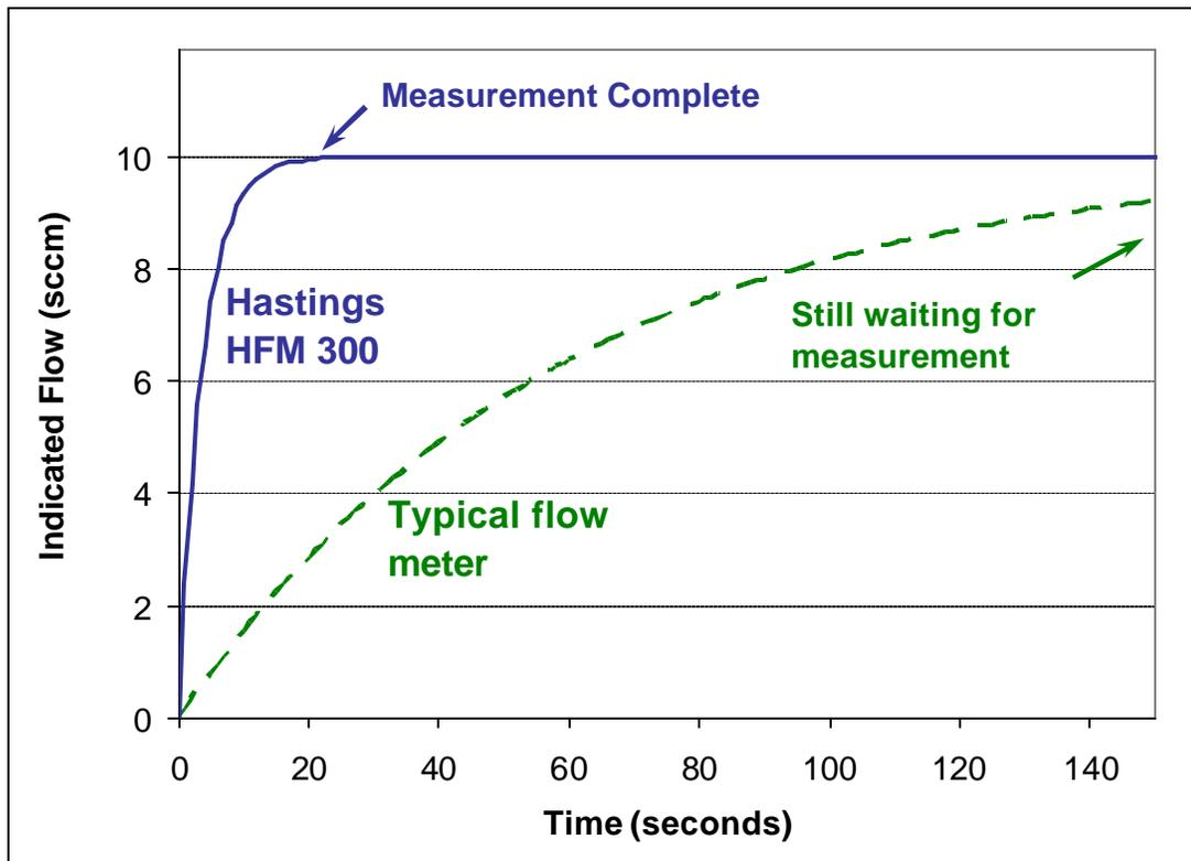
**By using the HFM 300, the time to accurately measure the leak rate (to within 2% of the final value) has been cut from over 4 minutes to just 16 seconds.**
