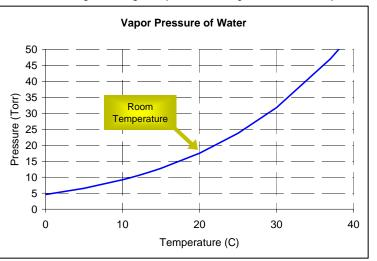
essentially useless in this application. However, an absolute vacuum gauge with high precision in the 0.01-20 Torr range can be effectively used to ensure proper evacuation has been achieved. The type of vacuum gauge most often used in this application is a thermocouple (TC) gauge.
