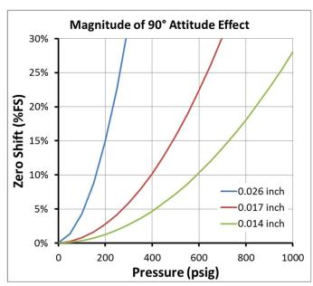
If the instrument is measuring light gases or low pressure, the change in the zero due to natural convection will be minimal. Larger shifts could be zeroed out with the zero pot as long as the upstream pressure is stable. A chart is shown here for nitrogen/air versus pressure.
