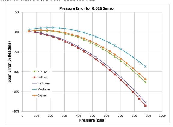
If the system pressure is higher than 250 psig (1.7 MPa) the pressure induced error in the span reading becomes significant. This error will approach 16% for nitrogen at 1000 psig. For accurate high-pressure measurements this error must be corrected.
