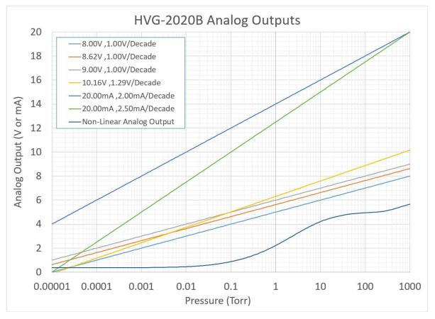
There are two other analog output options that are available. One is a non-linear curve based on convection gauges. The other is a dual slope output. These are described below.
