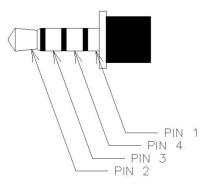
If making up a cable to interface from the TRRS 3.5 mm jack connector to a standard PC 9-pin serial port (RS232), use the connections as listed here.
