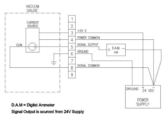
4 - 20 mA wiring diagram w/ unipolar supply
