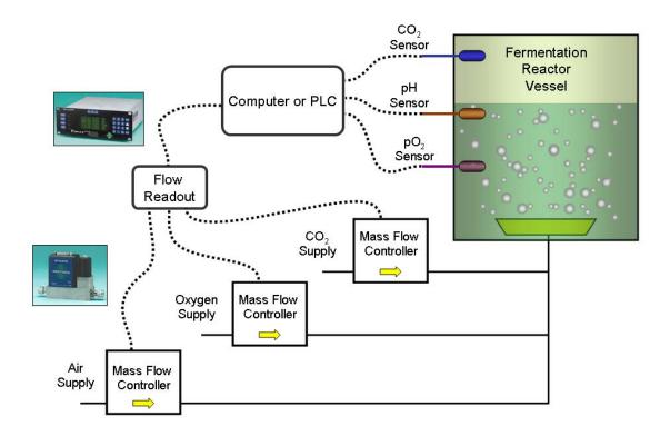
In this implementation a Flow Readout is used to interface (via RS-232) with the system's computer or PLC. The Flow Readout maintains individual set points to each of the mass flow controllers and provides other real-time functions such as event tracking, alarm status, and flow totalizing. This frees the system's computer from real-time flow monitoring and control.
